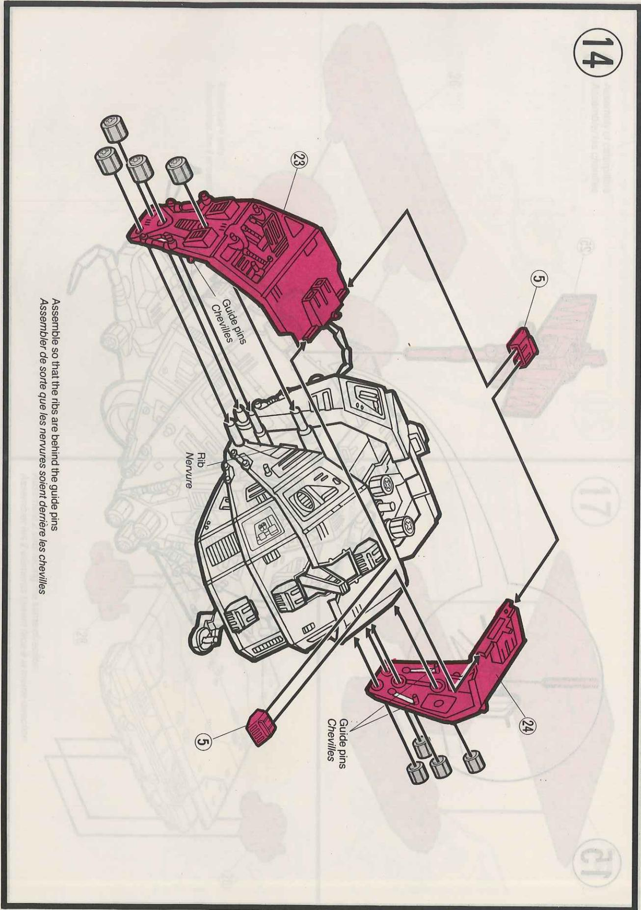
Assemble so that the ribs are behind the guide pins
