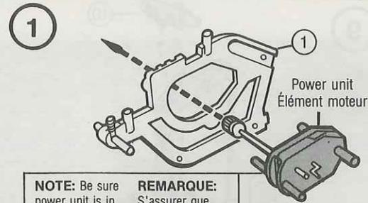
**NOTE:** Be sure power unit is in proper position.
